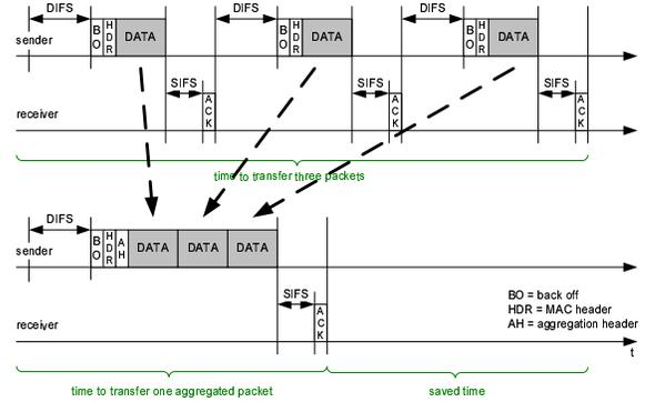
Fig. 3. Principle of Packet Aggregation
