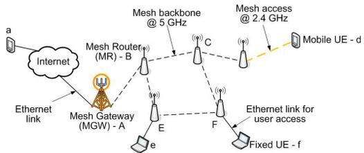
Fig. 1. MeshBed architecture
