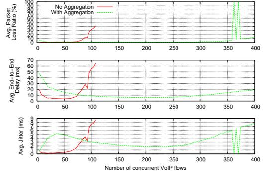
Fig. 5. PLR, delay and jitter of VoIP flows
