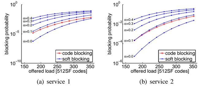
Fig. 3. Impact of orthogonality factor on the relationship of code and soft blocking
