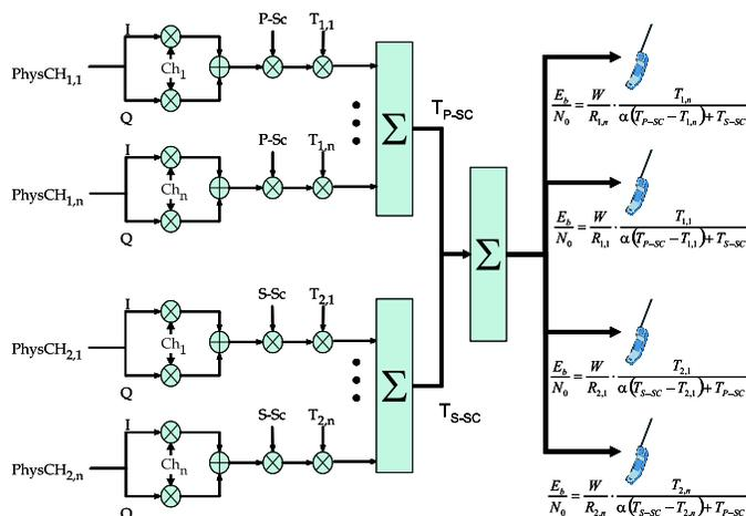
Fig. 1. Spreading and scrambling operation with primary and secondary scrambling code
