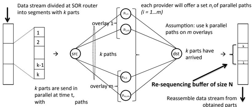
Figure 1: Transmission Mechanism
