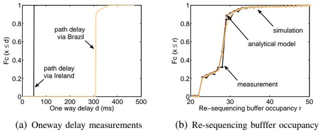
Fig. 1. Measured one way delays and resulting re-sequencing buffer occupancy for measurements, simulation and analysis
