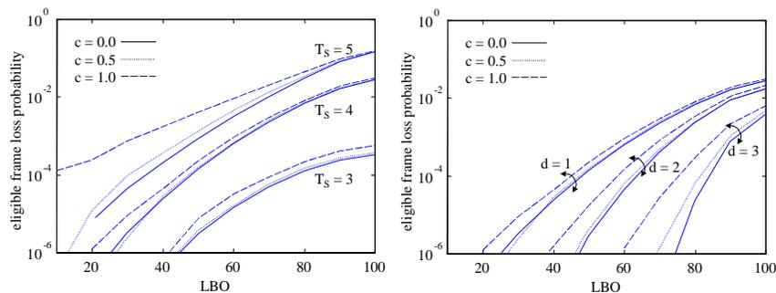
Figure 6: Influence of the available capacity and the traffic-streams burstiness.
