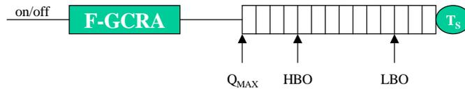
Figure 3: The basic GFR model
