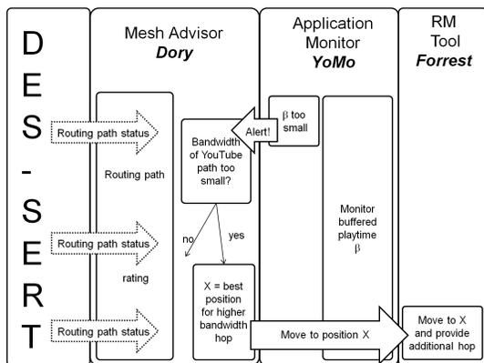
Fig. 1. Interaction of the components during the demo
