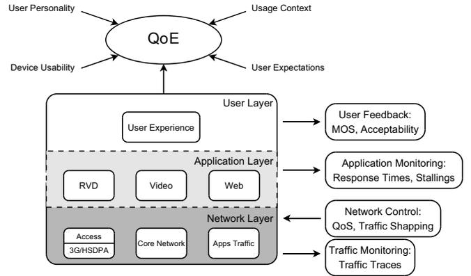
Fig. 1. Layered QoE evaluation methodology for networking applications.
