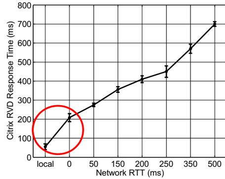
Fig. 4. Citrix response time. Even in optimal network delay conditions, Citrix RVD introduces an additional latency of about 150 ms w.r.t. a local desktop.
