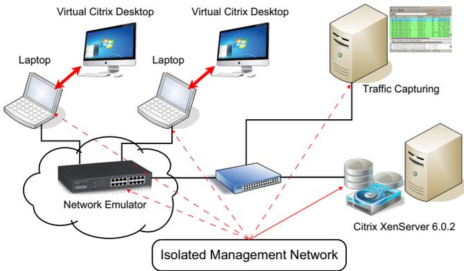
Fig. 2. Experimental testbed for subjective QoE testing of Citrix RVD.
