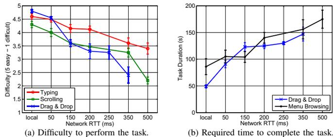
Fig. 6. Impact of RTT on user behavior and productivity. A RVD user may take up to 3 times more to complete a task in poor network conditions.
