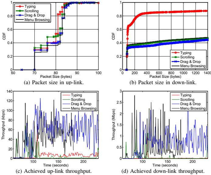
Fig. 3. Characterization of the traffic generated by Citrix RVD systems.
